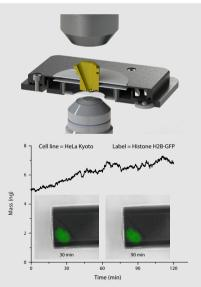
Optical microscope integration and full temperature, gas, and humidity control allow continuous monitoring of cells over a long period of time (up to days) with optical techniques (e.g. DIC, fluorescence) in addition to mass measurements. Images in graph show a time series of Histone H2B-GFP-labelled HeLa cells attached and growing on the Cytomass Monitor's cantilever. Data courtesy Müller lab ETHZ.
